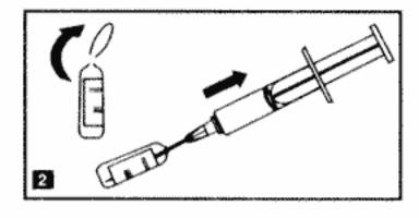
Break the top of the ampoule containing the solvent. Remove the plastic cover of the needle.
